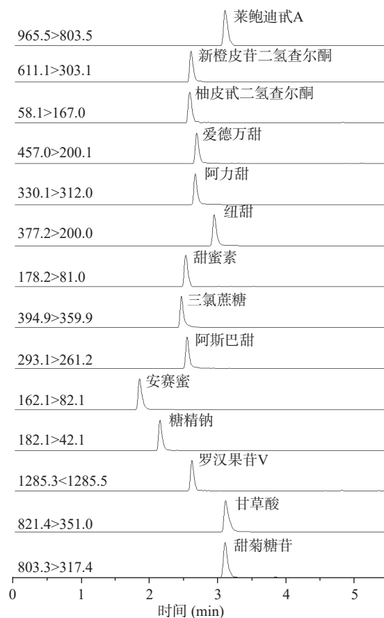
图1 14种甜味剂定量离子对的提取离子色谱图 Fig.1 Extracted ion chromatograms of 14 quantitative ion-pairing sweeteners
